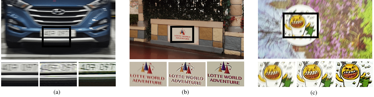
Figure 8. Image deblurring results. Blurred images are shown on top. In the bottom: original blurred image patch, deblurred result using [29] in sRGB space, and deblurred result in RAW space. Deblurring in RAW space outputs much sharper images.
